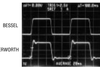
Figure 4. Oscilloscope of square wave response; top trace is the LTC1065 Bessel filter, bottom trace is the LTC1063 Butterworth filter
