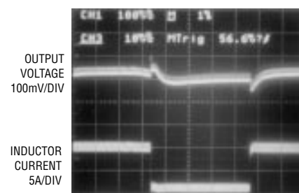
Figure 4. Oscilloscope showing effects of bidirectional loading on the GTL supply
